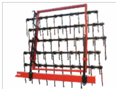
Spring harrow section with a heavy-duty tooth 16 mm (TTN)
