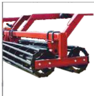
Press wheel two-row roller and three rows of small harrows
