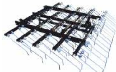
with a L-shaped spring tooth (weeder)
