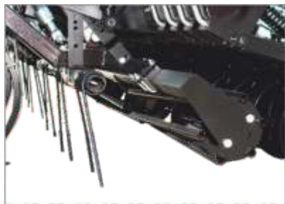
Damper unit (small harrow and roller)
